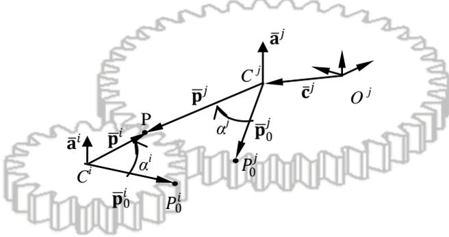
Figure 1: Spur Gear Joint
