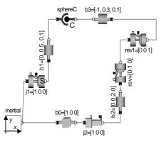
Fig. 2. Dymola model of the 4-bar pendulum
