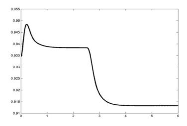
Fig. 4. Z-coordinate of the car body
